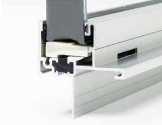
Milgard Thermally Improved Aluminum windows consist of extruded aluminum, where a “channel” is cut through the aluminum and polyurethane is poured into this channel to separate the interior from exterior extrusion. This process is done to reduce thermal transfer and improve energy efficiency.
