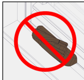
Incorrect Handle Install
