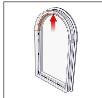
RT Head Cover Install
