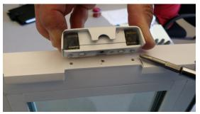
7. The screw holes may be stripped, if this is the case you will need to slide the stiffener bar over using the Phillips screwdriver.
