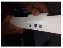
7. Using a Phillips screw driver, push the mortise lock body out of the vinyl frame.
