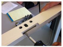
8. To reassemble, start by making sure the mortise latch is extended by depressing the release button at the side of the mortise latch.
