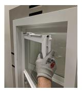
8. Put pressure on the left sash cam by pushing the panel into the left jamb. Without releasing the leftward force, swing right side of the panel toward the frame. If done correctly, the left sash cam will bend and allow the panel to clear the right side of the frame. The right sash cam should snap in with an audible click.
