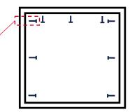
Product arrives with pre-drilled holes in covers & caps for fasteners; Drive QTY 9X #8-15 x 2" zinc coated flat head wood screws at pre-drilled locations flush with inner wall. Then cover clearance hole with cap.
