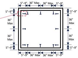
Drive minimum QTY 12X #8-15 x 2" zinc coated flat head wood screws through L bracket and into rough opening. Add additional fasteners as necessary to meet the spacing criteria.
