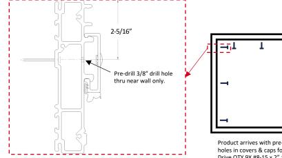
F Product arrives with pre-drilled holes in covers & caps for fasteners; Drive QTY 9X #8-15 x 2" zinc coated flat head wood screws at pre-drilled locations flush with inner wall. Then
