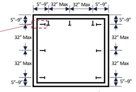
Drive minimum QTY 9X #8-15 x 2" zinc coated flat head wood screws at designated locations flush with inner wall. Add additional fasteners as necessary to meet the spacing criteria.
