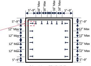
Drive minimum QTY 18X #8-15 x 2" zinc coated flat head wood screws at designated locations flush with inner wall. Add additional fasteners as necessary to meet the spacing criteria.
